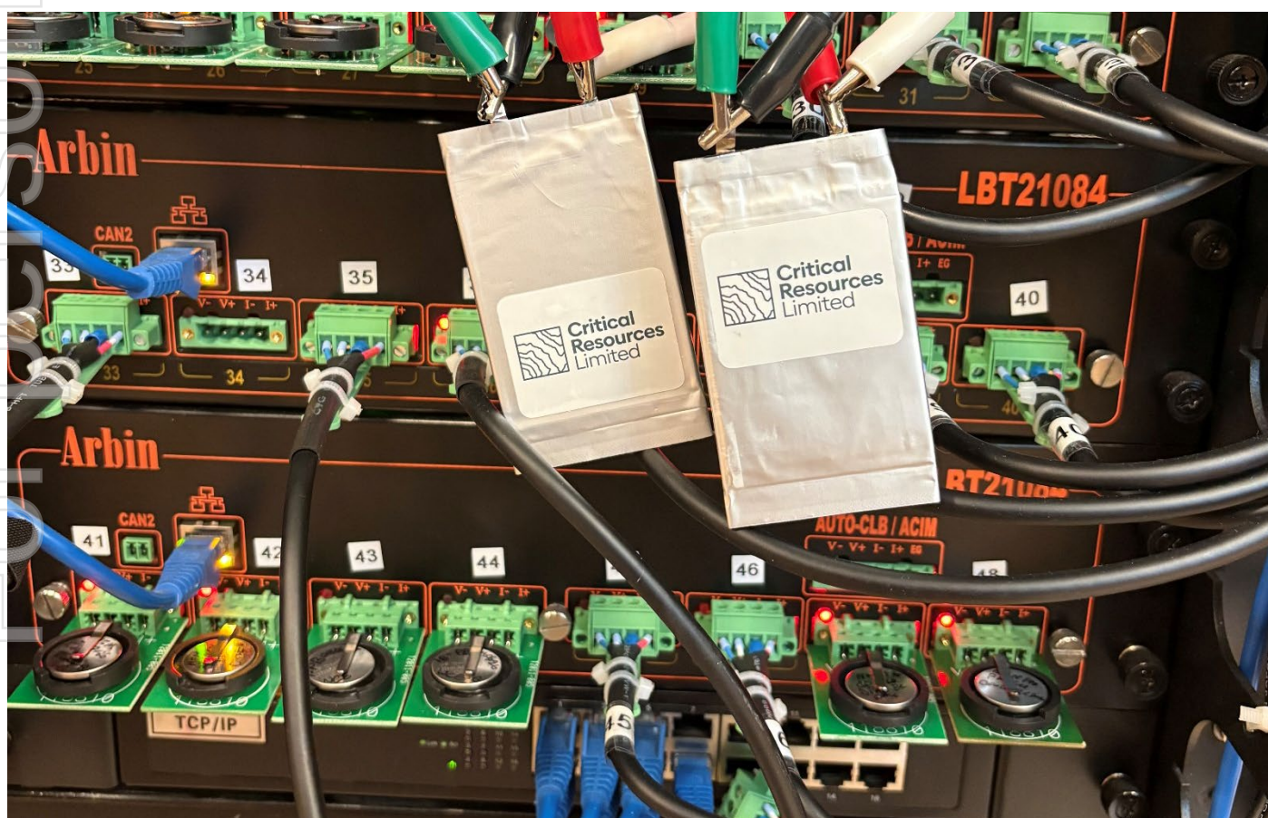
Figure 1 – The full-format DSD pouch cells under electrochemical testing
