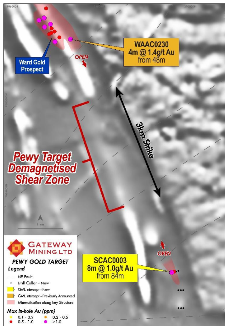
Figure 1: Demagnetised portion of the shear, highlighting Pewy.
