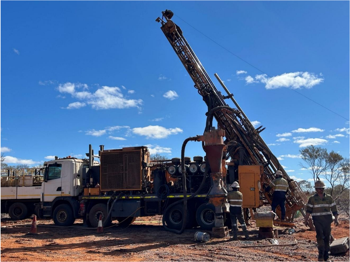
Figure 4: RC Drilling in action testing one of the six copper-gold targets at Juggernaut.
