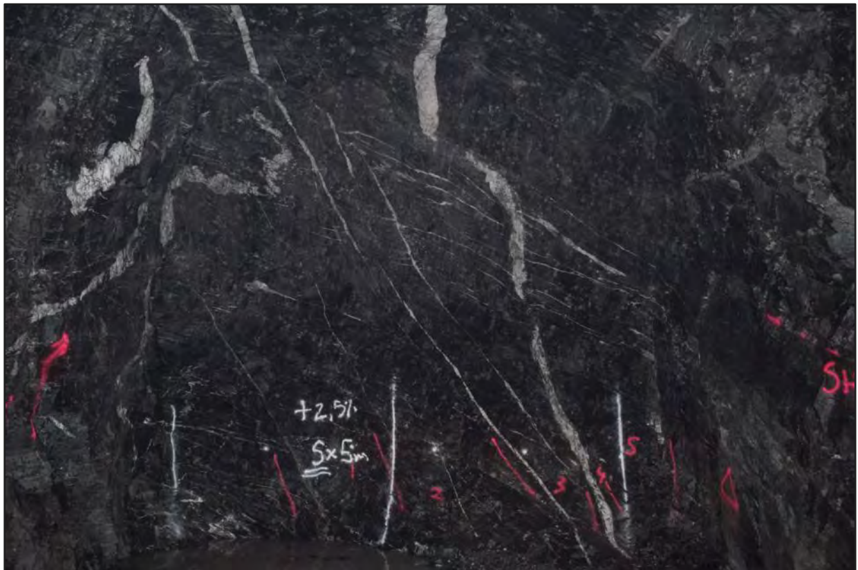
Figure 10-2: Underground Chip Sampling, Aurora Zone
