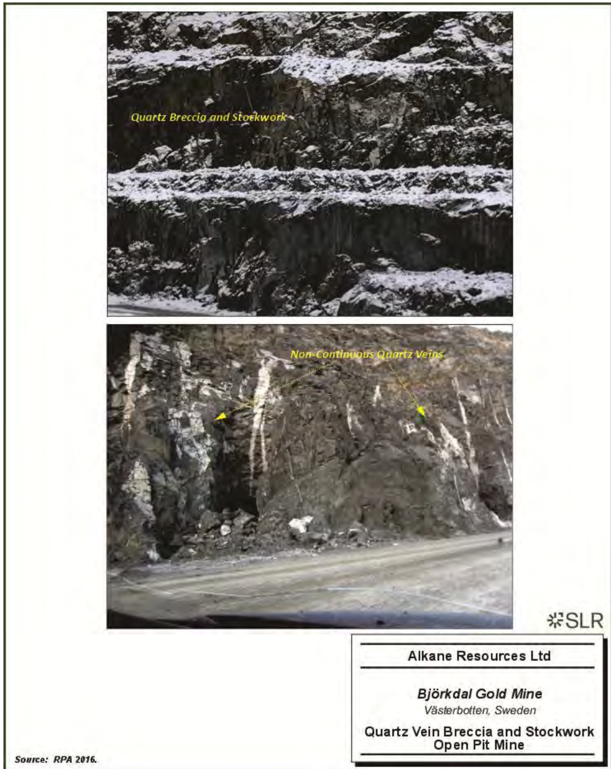
Figure 14-9: Quartz Vein Breccia and Stockwork, Open Pit Mine
