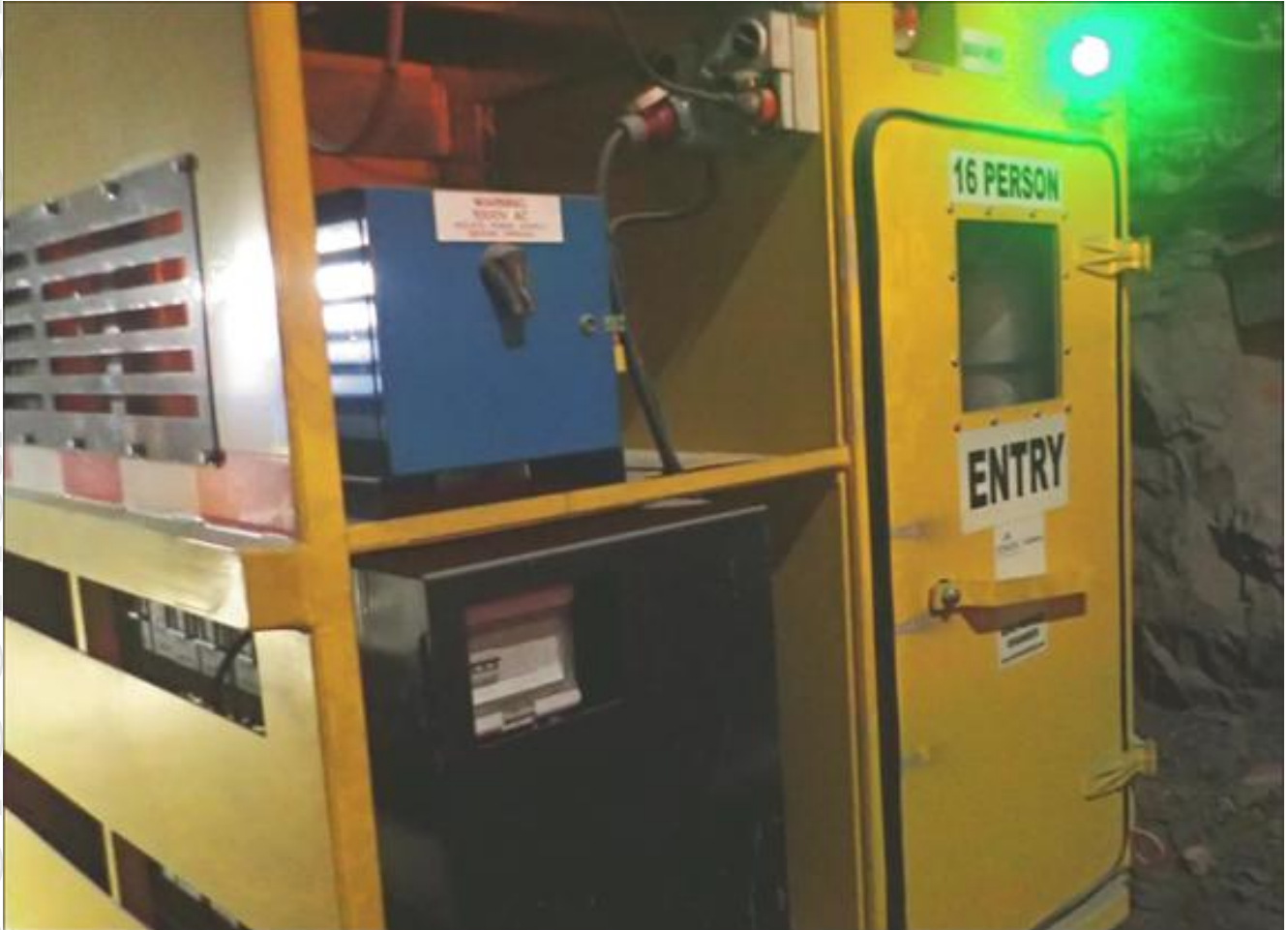
Figure 16-9: Typical underground refuge chamber
