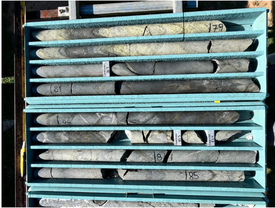
Figure 1. Diamond drill core from CMKNI011 showing 20–50 cm thick sulphide veins hosted within silica-sericite altered rhyolite, intersected within the interpreted Southern Lode at Silica Hill. The hole is still underway.
