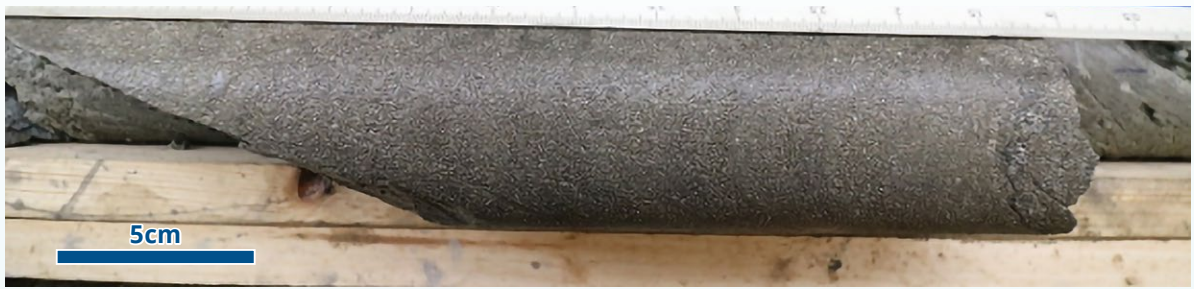
Figure 3: Example of massive sulfide from the Fuego Prospect (K26-571, 61.8-62.0m downhole). The interval from 61.0 to 62.0m returned assays of 126g/t Ag, 5.5% Zn, 0.9g/t Au, 0.1% Cu, 3.8% Pb.
