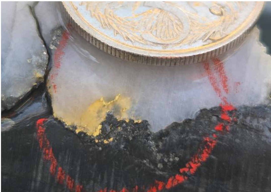
Figure 1 Visible gold in BMDD011W08 at 825.9m
