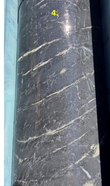
Photo 1 - 3: Grey metamorphosed sandstone with silica/sericite alteration with disseminated brassy pyrite throughout (1 - 5% Pyrite) with quartz carbonate bands (36.6m to 40.3m – BDDD002).
