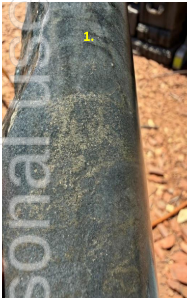
Photo 1 - 3: Grey metamorphosed sandstone with silica/sericite alteration with disseminated brassy pyrite throughout (1 - 5% Pyrite) with quartz carbonate bands (36.6m to 40.3m – BDDD002).
