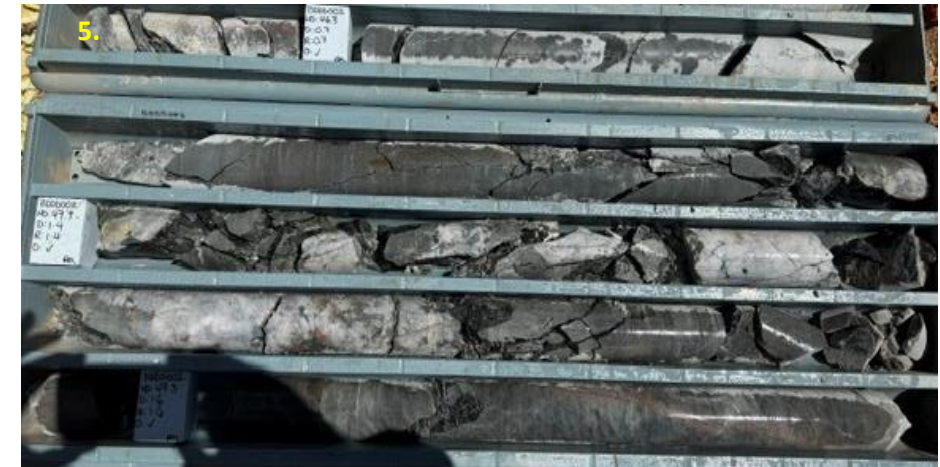
Photo 3 & 4: Banded pyrite and carbonations interbedded in fine grained mudstone with fine quartz veining is a classic signature of early diagenetic to hydrothermal sulphidic fluid activity in a low-energy sedimentary basin (79.9m to 82.5mm- BDDD002).
