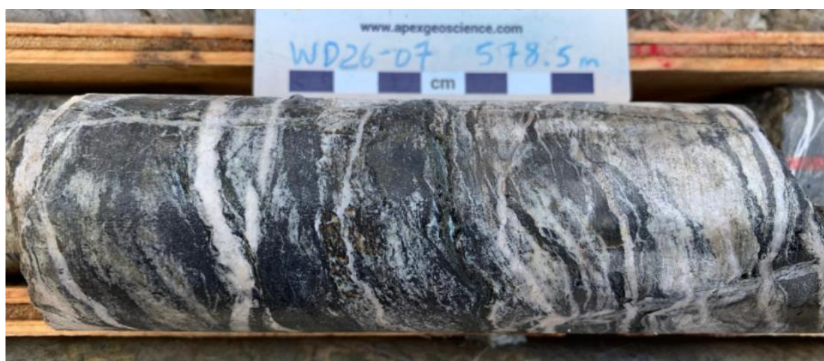
Figure 1: Very strong visual magnetite (black), sphalerite (brownish) and chalcocite (dark grey) bands within exo-skarn in NQ drill core from approximately 578.5m downhole in drill hole WD26-07. Laboratory assays for this interval are pending.
