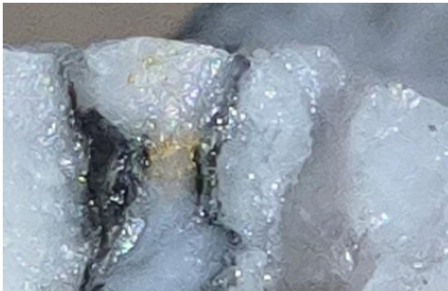
Figure 2. Visible gold 1 grains (lustrous yellow) up to 1mm and sulphide minerals in quartz veining in hole ATDD002 at 91.8m down hole. Core diameter 47.6mm. Assays are pending for this hole
