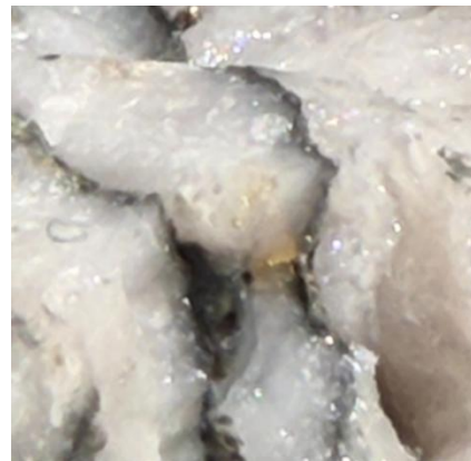
Figure 2. Visible gold 1 grains (lustrous yellow) up to 1mm and sulphide minerals in quartz veining in hole ATDD002 at 91.8m down hole. Core diameter 47.6mm. Assays are pending for this hole
