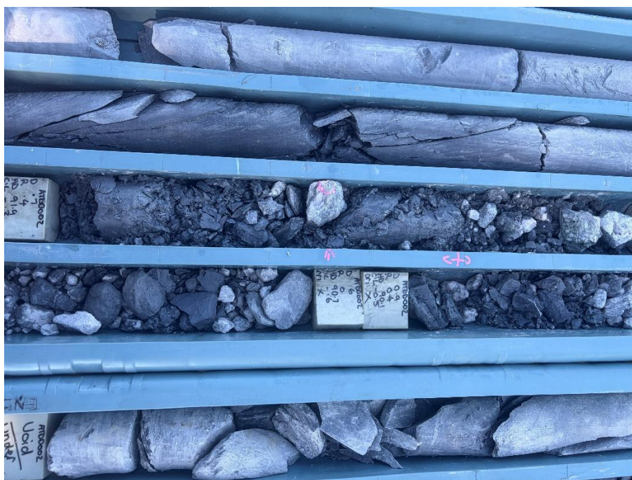
Figure 4. Drill core from ATDD002 for the drill run of 89m to 93.8m down hole showing the mineralised vein in context (pink arrow). Core diameter 47.6mm.
