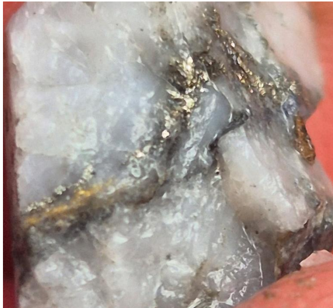
Figure 1. Visible gold 1 grains (lustrous yellow) up to 2mm and sulphide minerals, in quartz veining in hole ATDD002 at 98.1m down hole. Core diameter 47.6mm. Assays are pending for this hole.
