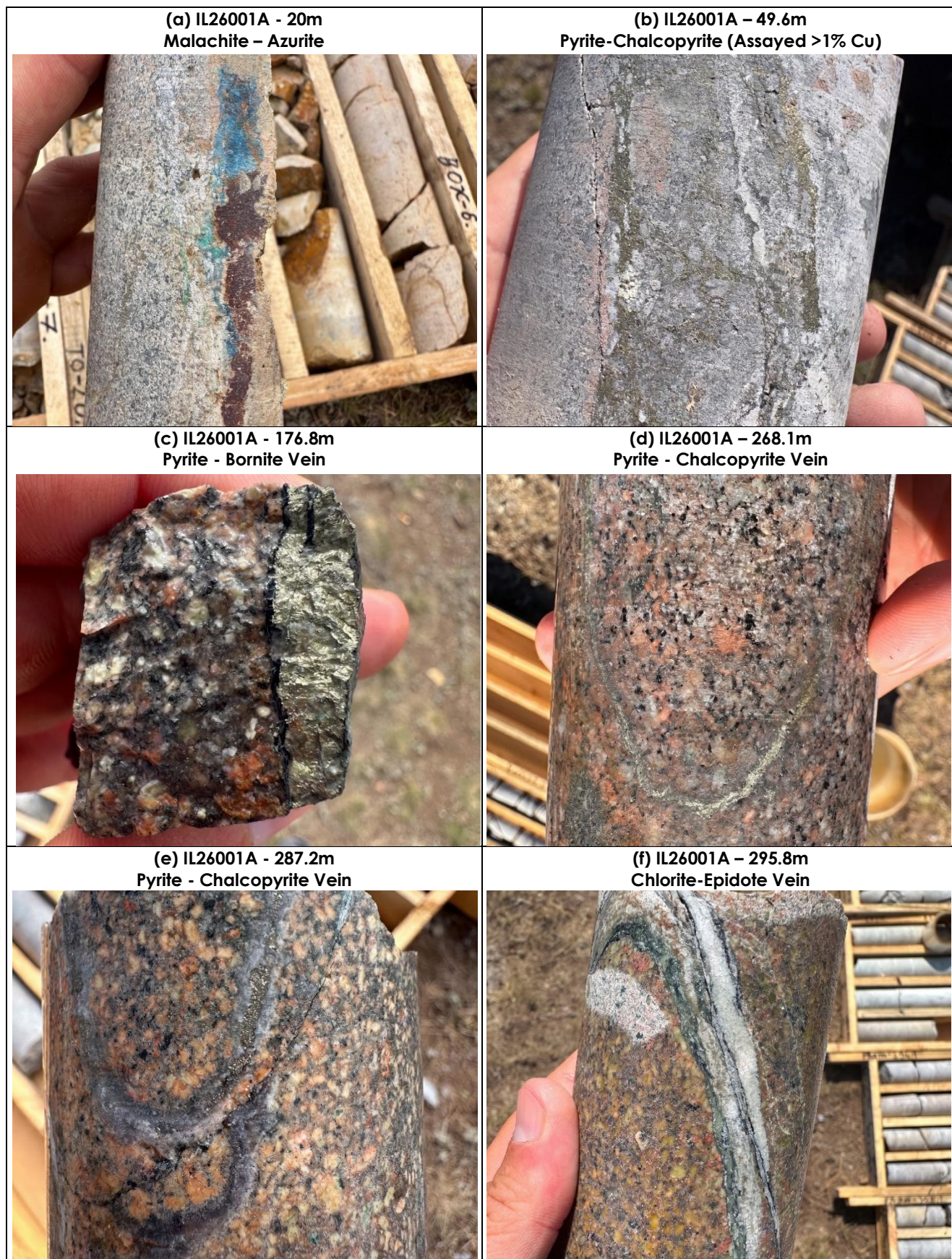
Figure 2 - Typical mineralisation and veining at Ilksan in hole DDH-IL26001A
