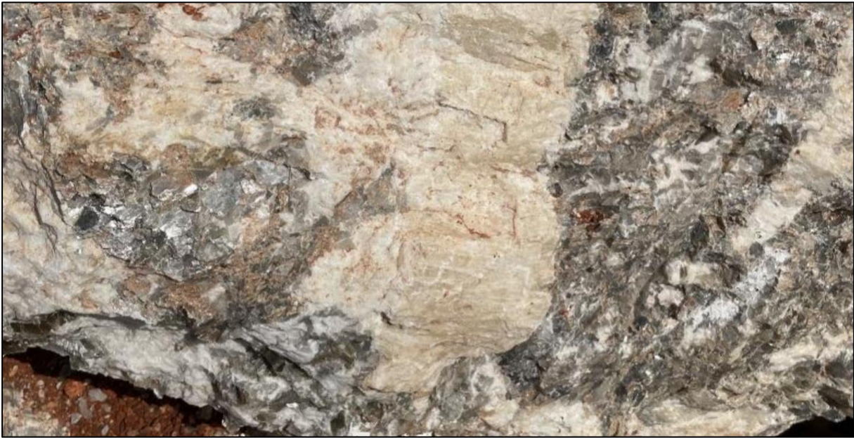
Figure 5: Pippingarra Project Hand specimen showing flake mica (grey), with potassium feldspar (cream), albite (white) and quartz (grey).
