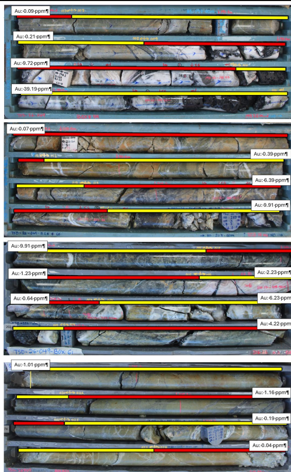
Figure 3: Mineralised structural zone in drill core from the 120 Vein (hole TSD-26-049), including 1 m at 39.19 g/t Au. The updated estimate captures the full width of zones like this, rather than a single narrow vein (HSC, September 2026).
