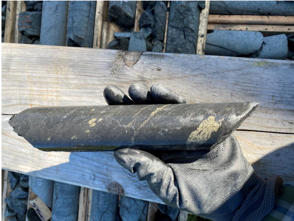
Photograph 3: Tillex Project TX26-007 drill core at 184.9m, disseminated, fracture fill and coarse chalcopryrite within argillite – assays returned 3m @ 0.45% Cu and 3.3g/t Ag from 182m
