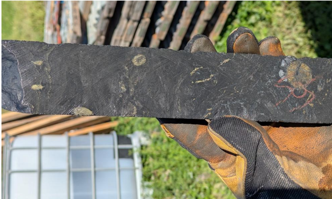
Photograph 2: Tillex Project TX26-006 drill core at 95m, disseminated and coarse chalcopyrite with minor quartz carbonate veining within argillite – assays returned 14m @ 1.38% Cu and 5.0g/t Ag from 83m
