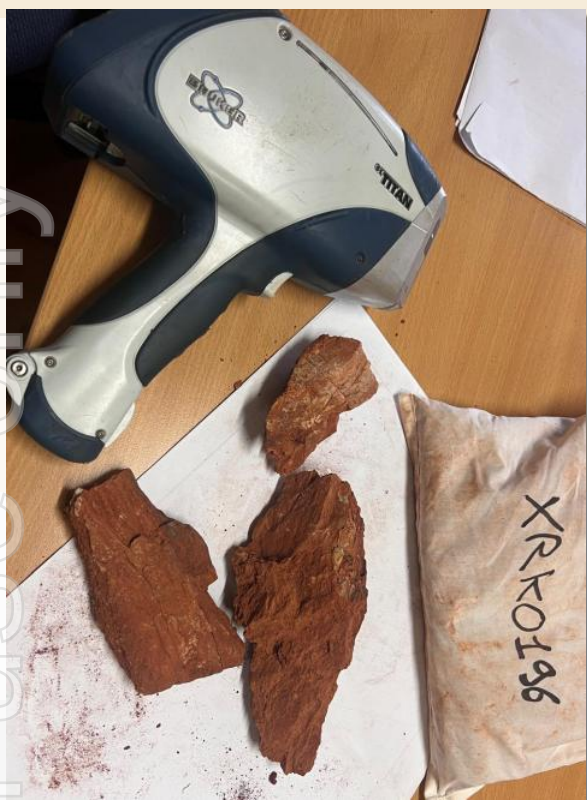
Picture 1: Rock Chip XRK0196 Ferruginous Copper Gossan
