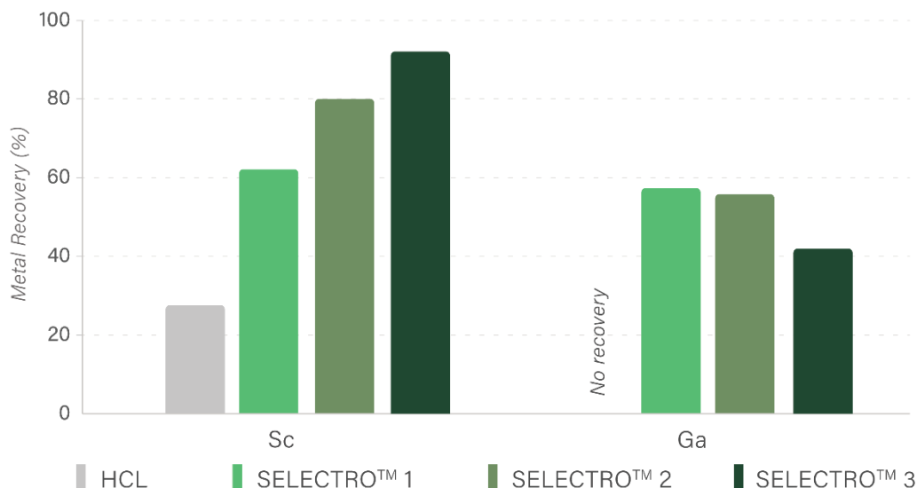
Figure 3: Scandium and gallium recovery by processing method, HCL baseline versus Selectro™ 1, 2 and 3.
