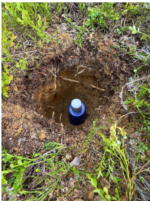
Figure 3: RadonX™ field deployment. Each inverted detector cup was buried in a shallow hole, its location recorded by GPS and marked with flagging tape, and recovered approximately 10 days later for field analysis.
