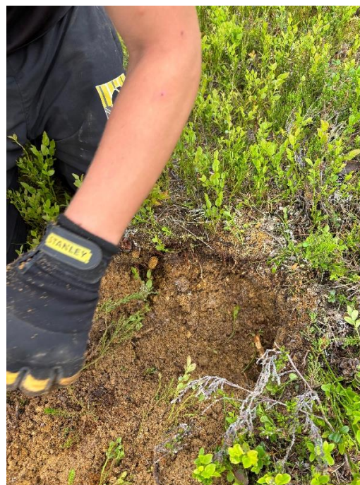
Figure 3: RadonX™ field deployment. Each inverted detector cup was buried in a shallow hole, its location recorded by GPS and marked with flagging tape, and recovered approximately 10 days later for field analysis.
