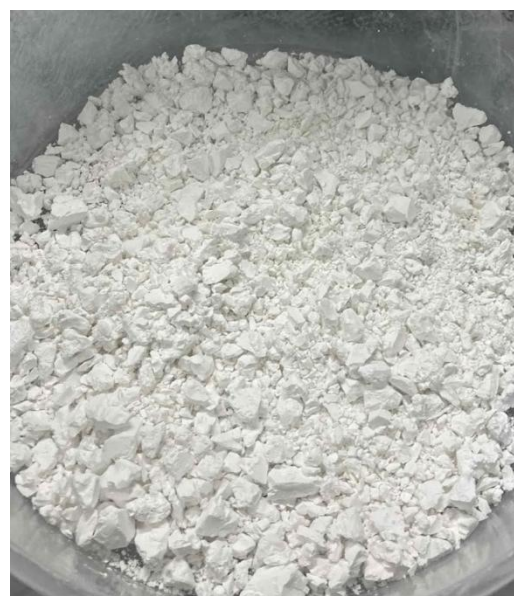
Figure 6: Hydrated niobium oxide precipitate (before calcination)
