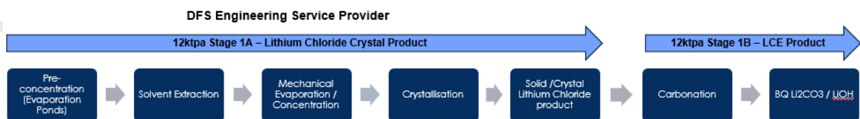
Figure 1. Rincon Lithium Project – Process Flowsheet
