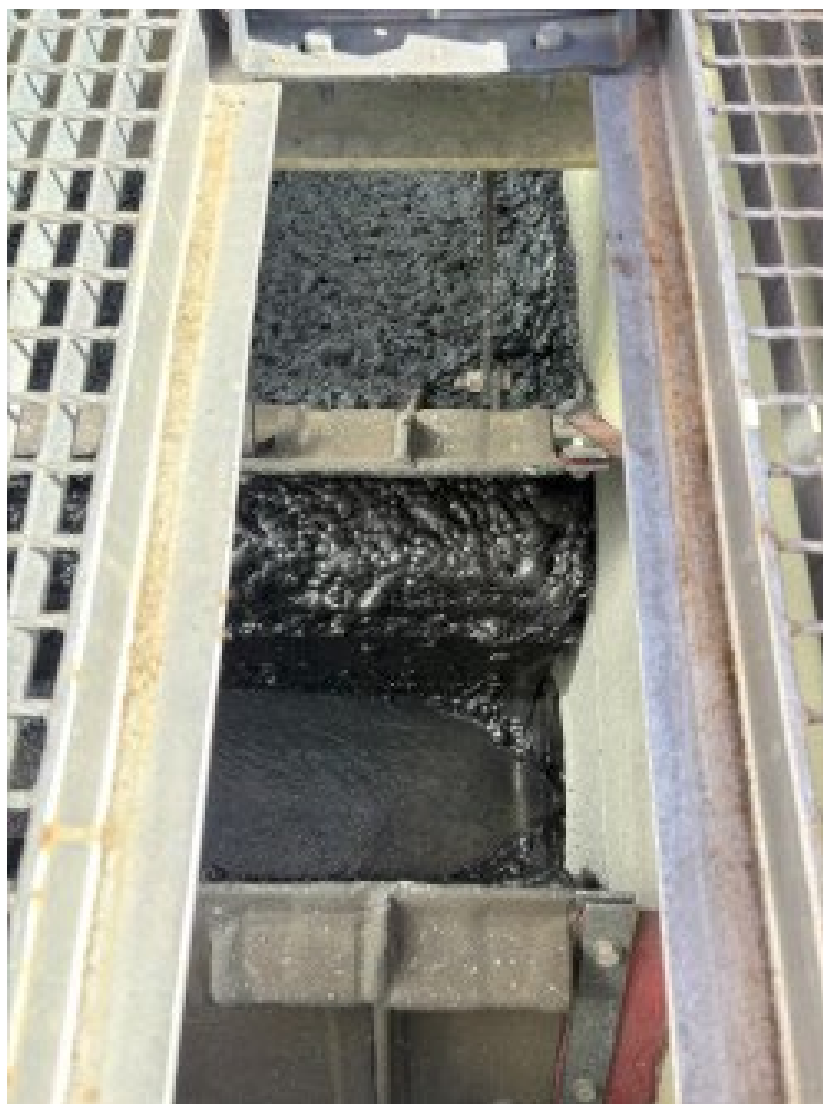
Figure 1 Antimony rougher flotation cells producing concentrate
