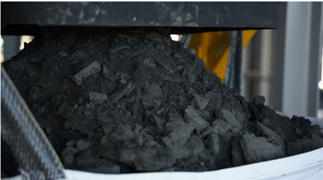
Figure 3 Concentrate produced after moisture removal by filter presses
