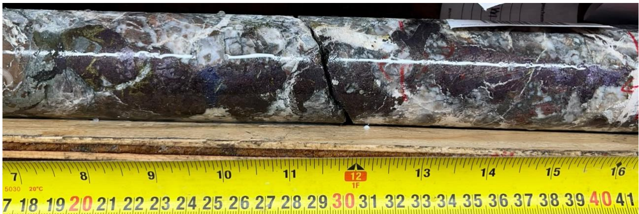
Figure 01 - Photograph of coarse-grained bornite-chalcopyrite mineralisation within a multiphase vein and breccia system at Bornite Hills. Photo of mineralisation from 83.7-83.9m in BNH26003.
