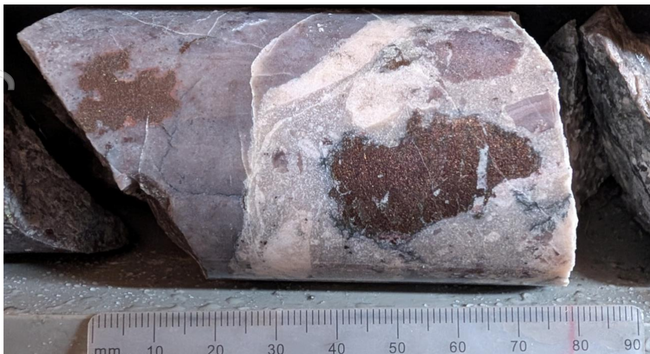
Figure 03 - Photograph of centimetre-scale bornite aggregates within a quartz-carbonate cemented breccia. Mineralisation characteristic of between 60.5-72.0m downhole in BNH26001A.
