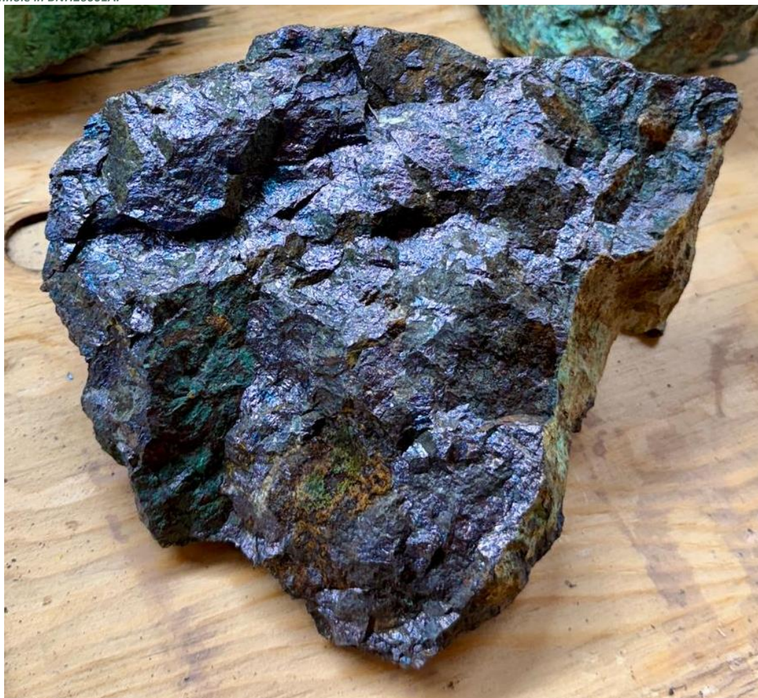
Figure 04 - Example of massive bornite from Bornite Hills showing. Rock is composed of >95% bornite with 1-3% chalcopyrite and accessory quartz-calcite. Sample is approximately 20cm across. Sample taken from NAD83/UTM Zone 11N 505699 E, 7501746 N. See announcement "Strategic acquisition of Bornite Lake prospect at Rae" 2 November 2025.
