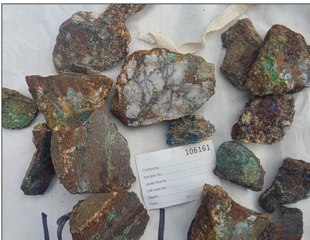
Figure 5. Sample No. 106161, brecciated milky white vein quartz with limonite, malachite and minor azurite; assay result 2.22 ppm Au, 0.2% Sn and 1.3% W. (FOV 25cm)
