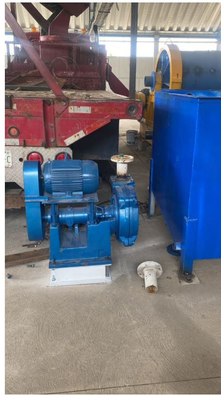
Figure 4: Cyclone box tower (left) and 3 x 3 SRL slurry pump delivered to site (right)
