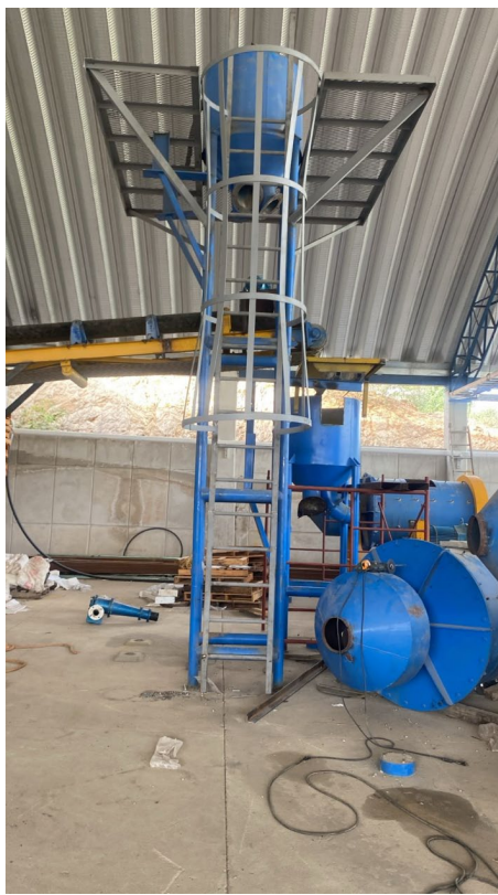
Figure 4: Cyclone box tower (left) and 3 x 3 SRL slurry pump delivered to site (right)
