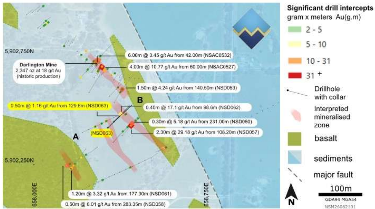
Figure 3 Plan view highlighting the strong continuity of the strike extension between drill holes.
