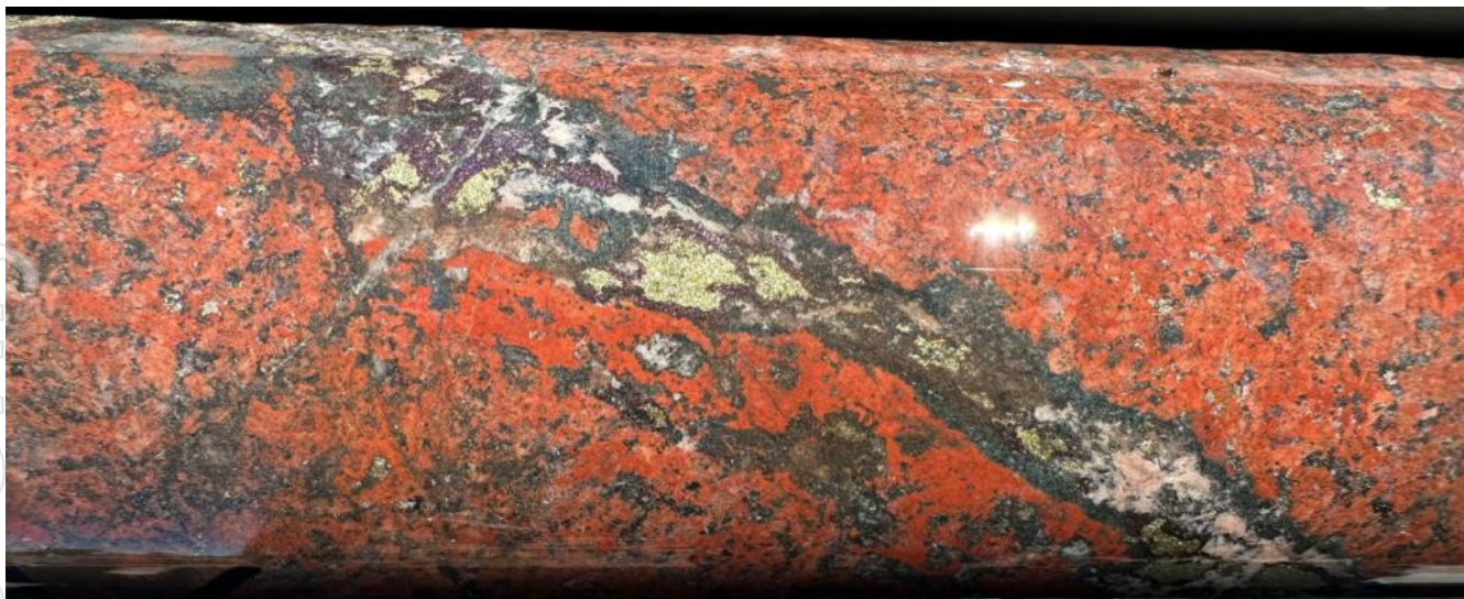
Figure 34: Carbonate-bornite (purple)-chalcopyrite (yellow)-specular hematite (dark grey) vein and disseminated chalcopyrite and bornite (purple) from 1,074 m – 1,074.15 m
