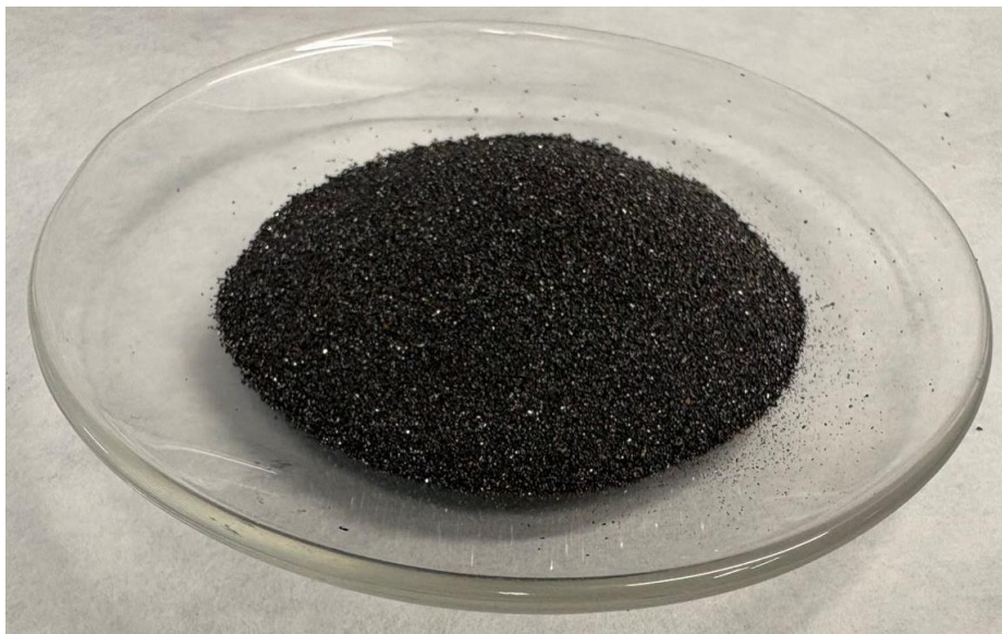
Figure 4: Mkanda rutile product +96% \text{TiO}_2
