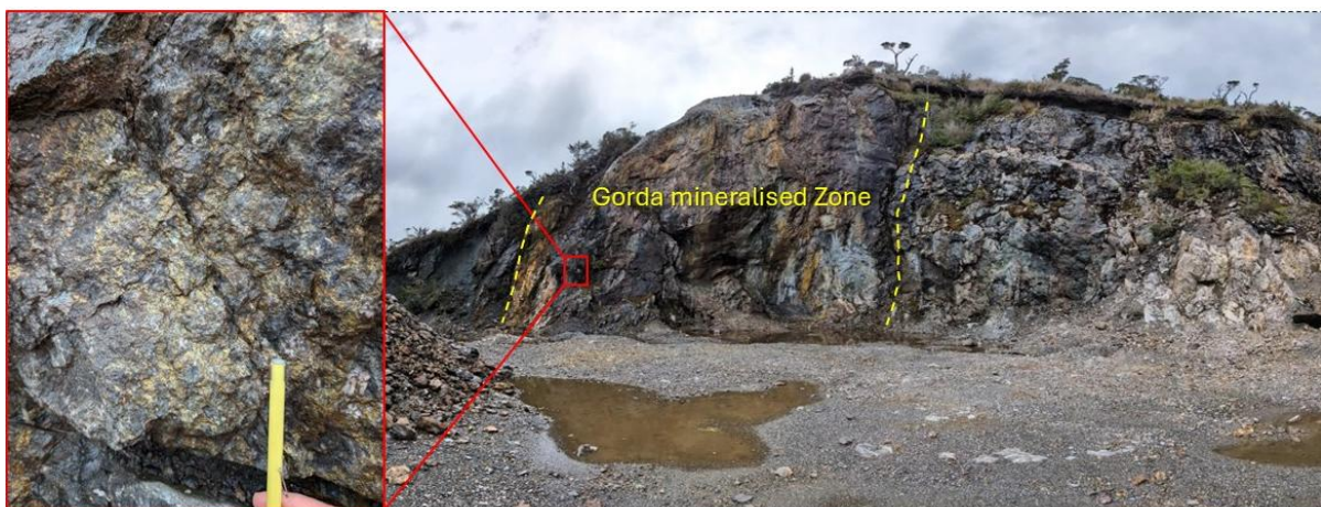
Figure 14. Quarry of the Gorda mineralised zone (~5m width), with insert showing chalcopyrite-quartz breccia hosted in Palaeozoic basement shale. Chalcopyrite estimate of 20% composition (Location 670,495m E, 4,085,504m N).
