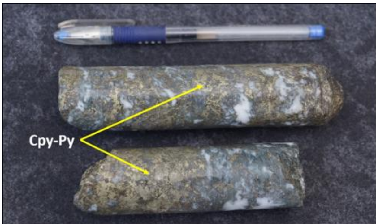
Figure 1. Quartz-chalcopyrite breccia mineralisation from 29Metals 2022 short drill program, core CUL56-583 3 . This sample returned 8.0% Cu, 214 g/t Ag and 0.2 g/t Au. Drilling shows potential vein extension, located ~600m north of the Cutter Vein working.
