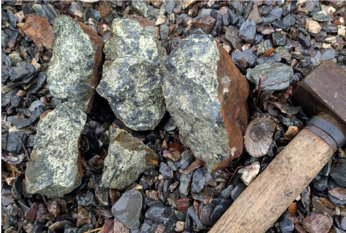
Figure 13. Massive sulphide quartz breccia ore from the stockpiles at the Cristina Central workings. Major sulphide phase is Chalcopyrite-pyrite, which averages over 50% in composition. Sample Submitted for assay, with results expected in ~3 weeks (sample location 670,256m E, 4,086,325m N).
