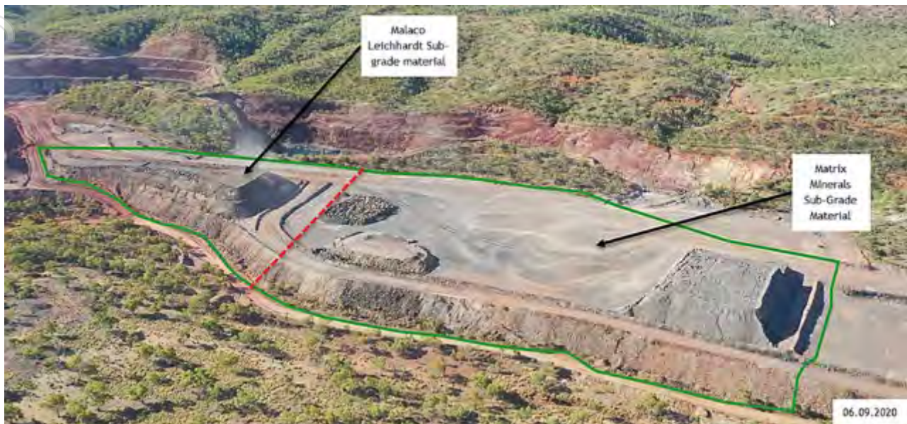
Figure 10-13. View of the ROM pad and extent of the Matrix and Malaco low-grade stockpiles, August 2020.
