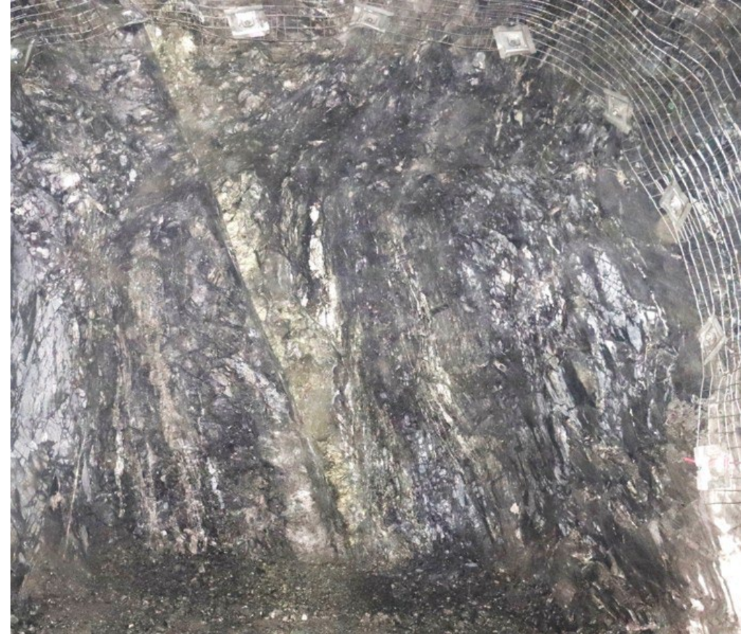
Development face look south along Jolly shoot development drive (on 5000L South), showing visible copper sulphide mineralisation. Face dimensions are approximately 5.5m wide by 4.9m high 2
